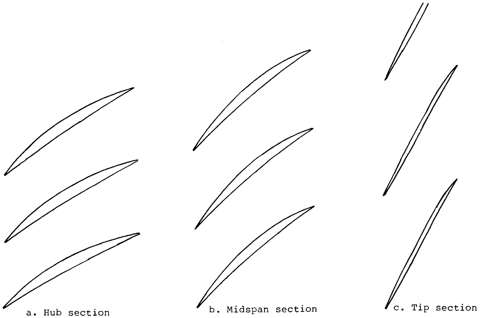
Figure 4. Typical blade sections of NASA low-aspect-ratio rotor.
