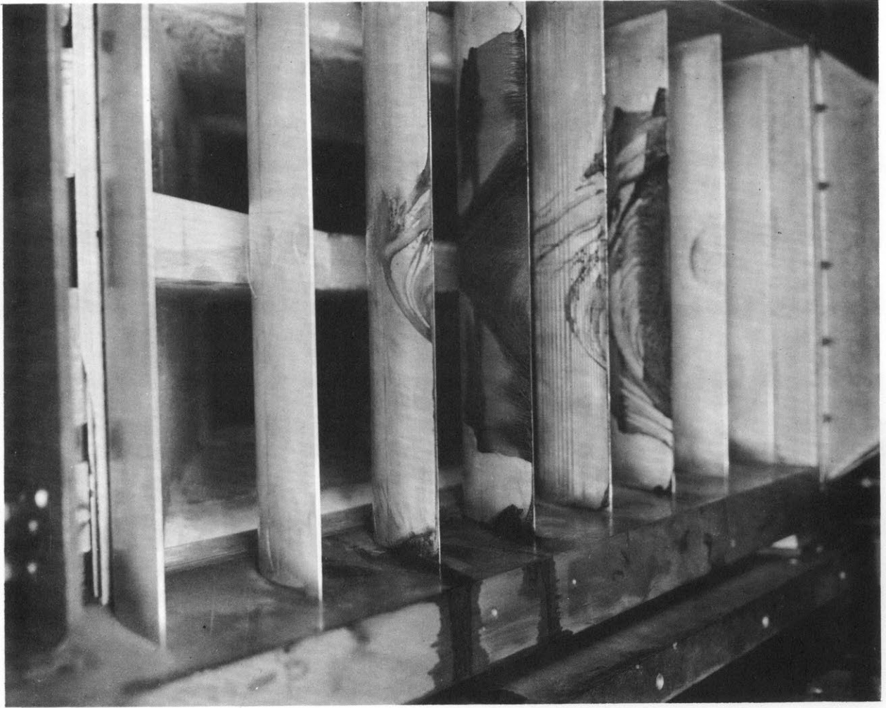
FIGURE 68 SKEWED WAKE FLOW. STREAMLINE TRACES IN CARBON BLACK ON THE BLADE SUCTION SIDE.
