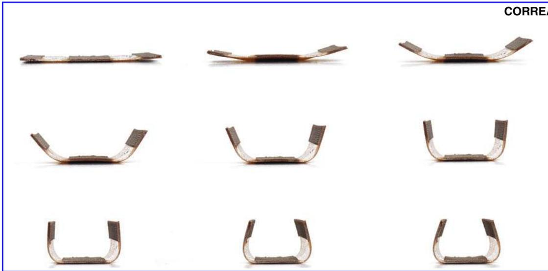
FIG. 5. A series of photographs showing a multimaterial printed wood composite developed by SAL that self-transforms from a flat sheet into a symmetrically folded structure.
