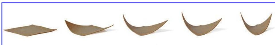
FIG. 4. A series of photographs showing a differentiated printed wood composite developed by SAL that self-transforms from a flat sheet into curved surface.
