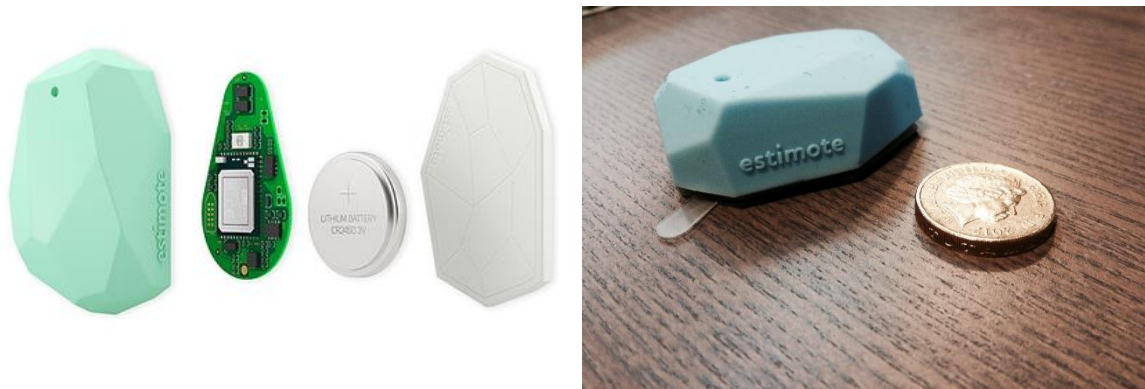
Figure 4.7 - Estimote beacon size and construction
