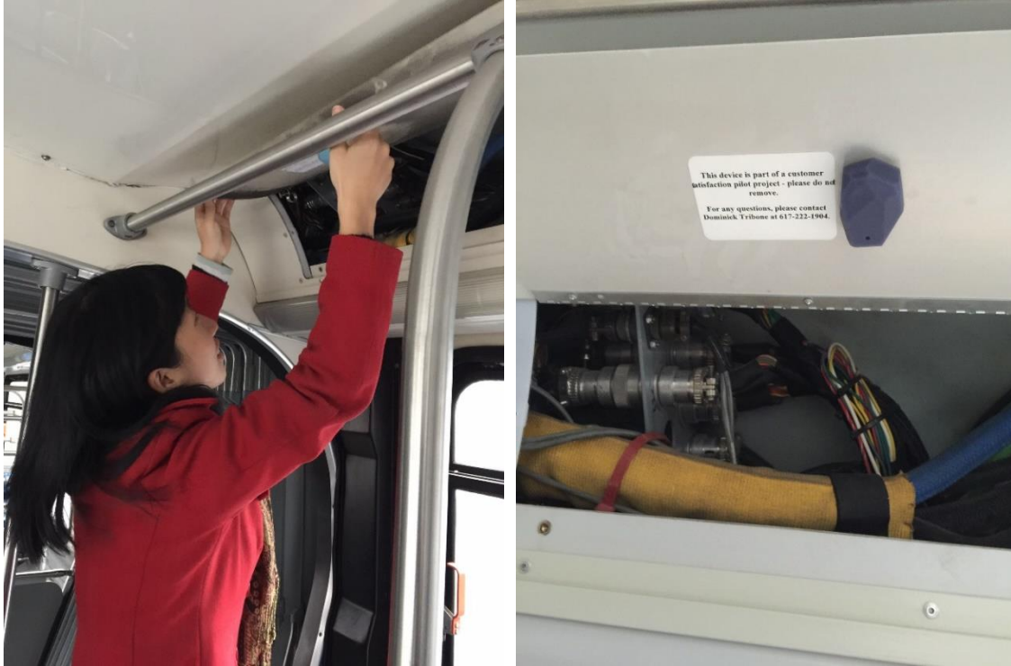
Figure 7.7 - Installing beacons on the buses
