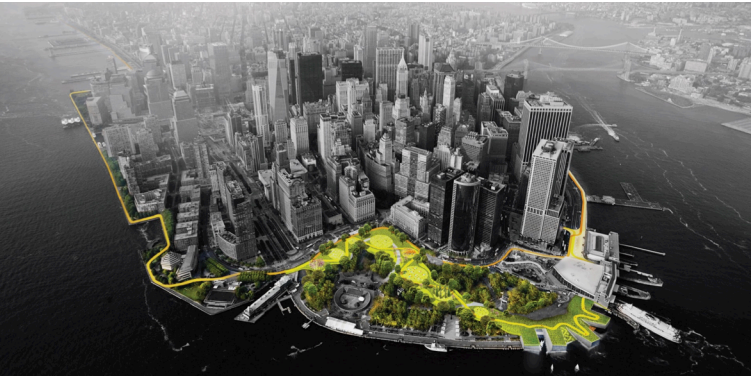
Fig. 1-2: The Big U, a winner of RBD, envisions the construction 10 miles of protective infrastructure around Lower Manhattan. Source: RBD.
