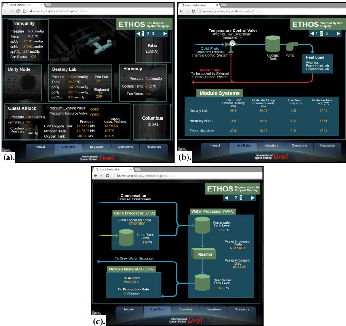
Figure 4-4: The three ETHOS console displays [160] (a). Atmospheric pressure, temperature, and composition within the ISS USOS (b). ISS USOS Active Thermal Control System (c). ISS USOS Regenerative ECLS Technologies
