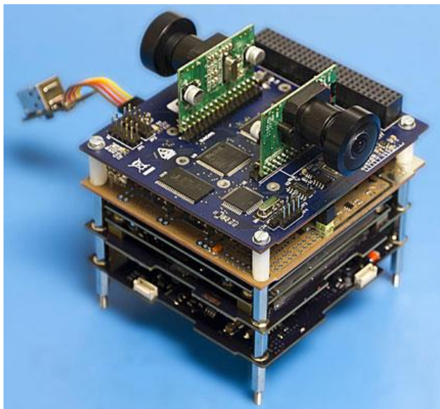
Figure 3: Example of an avionics “stack” 5
