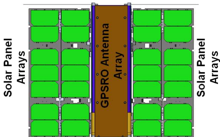
Figure 8: MiRaTA spacecraft design overview, back face 12
