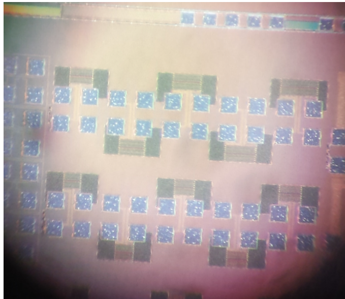
Figure 3-10: Some fabricated NMOS transistors in a variety of sizes
