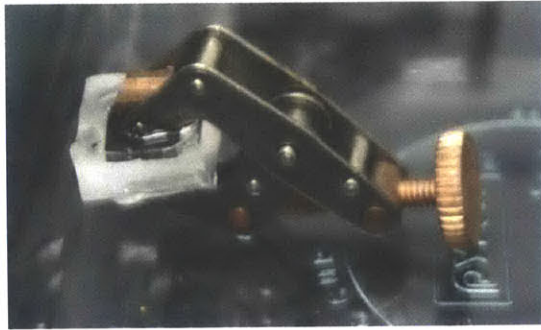
Figure 3-10 – C-clamp holds together the carbon substrate and the PDMS mold
