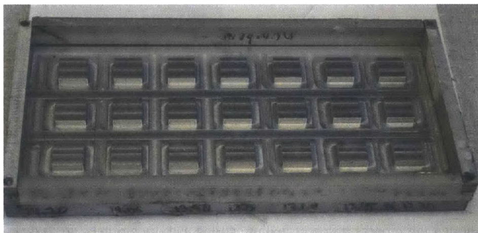
Figure 3-5 – Aluminum mold used for creating the PDMS mold
