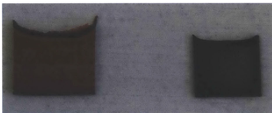
Figure 3-4 – Xerogel substrates: left side - RF xerogel substrate with meniscus forming at the contact of RF solution, PDMS mold and air; right side – the same substrate after pyrolysis
