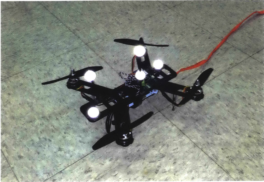
Figure 4-2: Example array of Vicon dots rigidly attached to a QAV250
