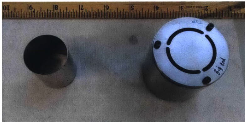
Figure 3-7: Left: One of the optics measured in this study, measuring about 1.75 inches long and 1.25 inches in diameter. Right: The stainless steel mounting structure designed for optics of this size, which holds the optic in place during alignment and measurement. The annulus of the structure allows x-rays to impinge on the optic while blocking the straight-through beam.
