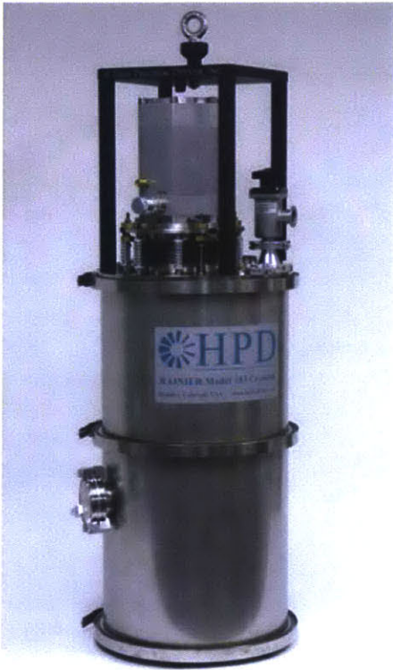
Model 103 Rainier ADR cryostat showing vacuum jacket, side port, pulse-tube head and anti-vibration bellows.
