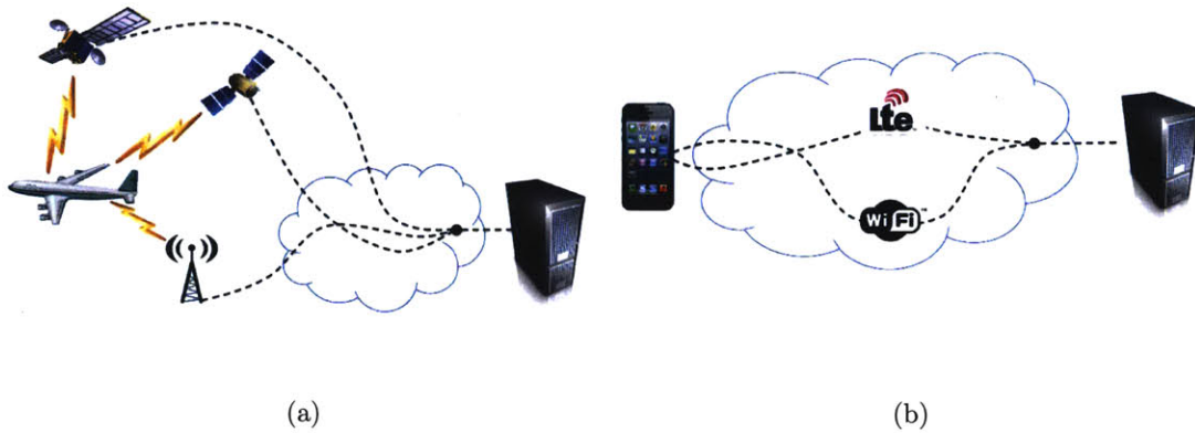
Figure 3-1: Simultaneous use of multiple heterogeneous networks can: (a) help to provide an increased quality of service to disadvantaged users, or (b) help to reliably offload traffic from one network to another.
