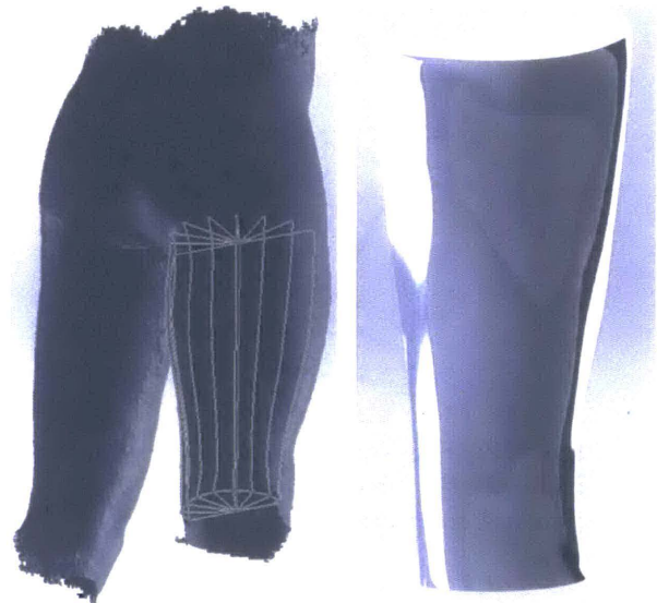
Figure 4: The STL file is traced with splines (left) and the profile is lofted to create a smooth and accurate part (right).
