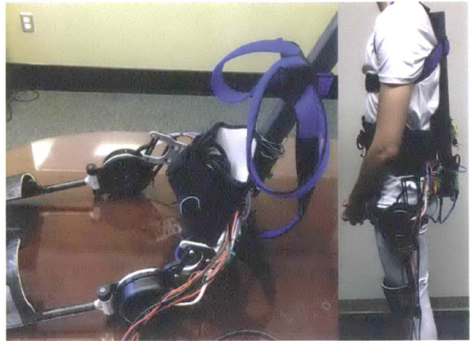
Figure 1: The alpha prototype of a dynamic human exoskeleton.
