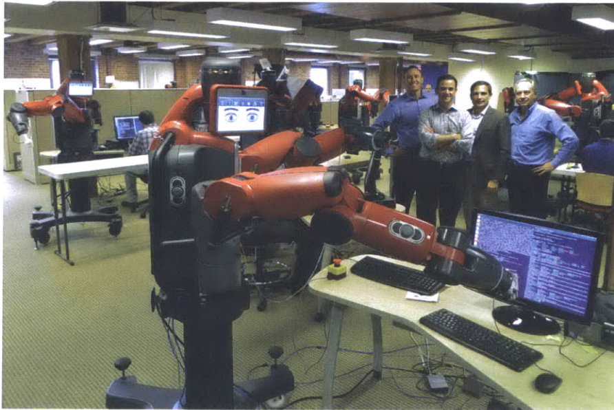
Figure 1.2: The Baxter robot created by Rethink Robotics can safely operate near human workers[3]. Its series elastic actuators and torque control allow it to stop upon making unexpected contact with human without causing injury. [5]
