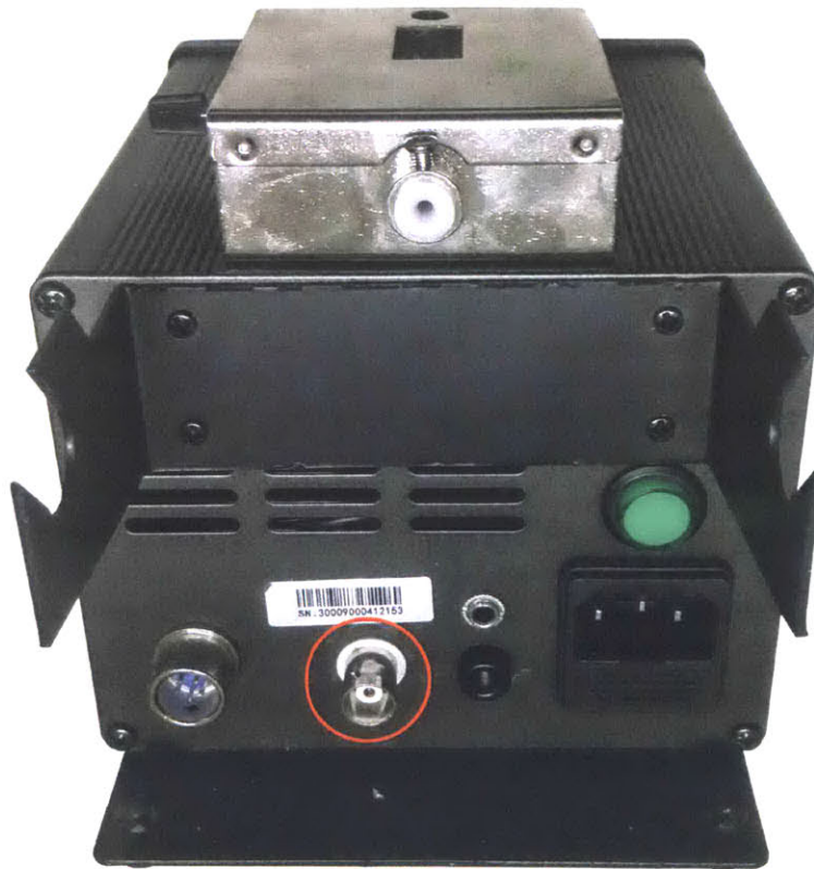
Figure 2.5: The BNC connector circled in red was added to the soldering station unit. It was connected in parallel to the existing K-type thermocouple embedded in the tip of the soldering iron. This allowed the temperature of the soldering iron to be measured without the need for an additional sensor.
