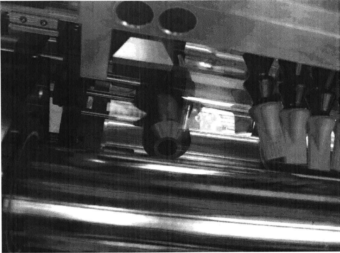
Figure 2.7: Microscope lens behind contact of glass and steel rollers
