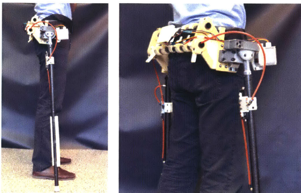
Figure 3 Wearing a prototype of the SRL. The SRL augments a user with two robotic limbs that are kinematically independent from existing limbs. In this prototype, a 3-D printed carbon fiber/Kevlar/nylon composite base, hollow carbon fiber limbs, and lightweight pneumatic cylinders are utilized to reduce overall mass and volume. Image credit Federico Parietti.
