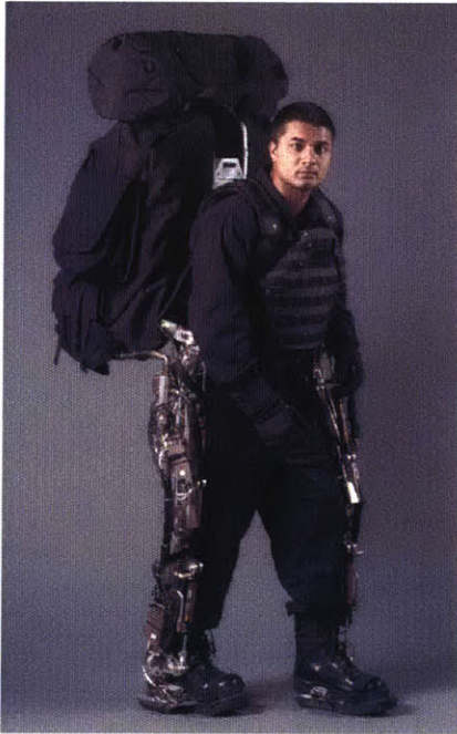
Figure 1 Berkeley's BLEEX (Lower Extremity Exoskeleton), designed for carrying heavy loads. This is an example of a conventional exoskeleton where motion is constrained to the natural motion of the user's limbs (in this case, the legs). Image credit Prof. Homayoon Kazerooni.
