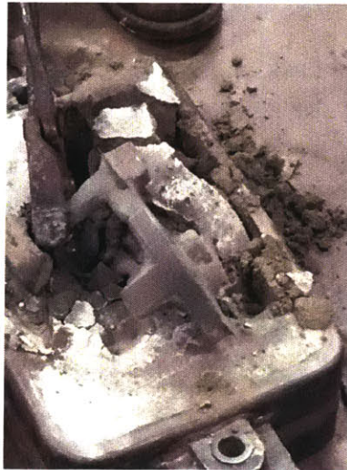
Figure 15: After metal has been poured and the part has cooled it is removed from the sand.
