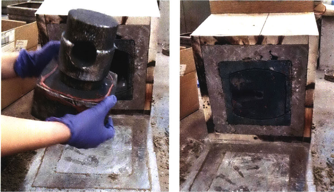
Figure 32: The core print was cantilevered into the flask and then the flask was moved onto the base and iron was poured.
