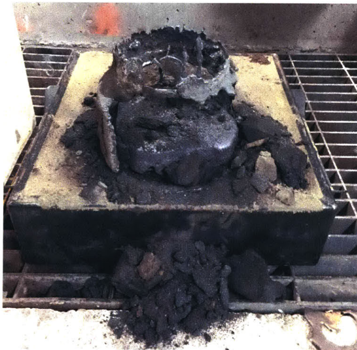
Figure 21: The failed piston. The core collapsed and the iron filled the hollow part of the core print.
