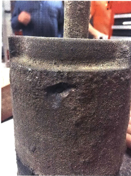
Figure 35: A void appeared on the piston. It is located in the vicinity of the piston rings so it should be mostly bored out and should not affect the piston performance.
