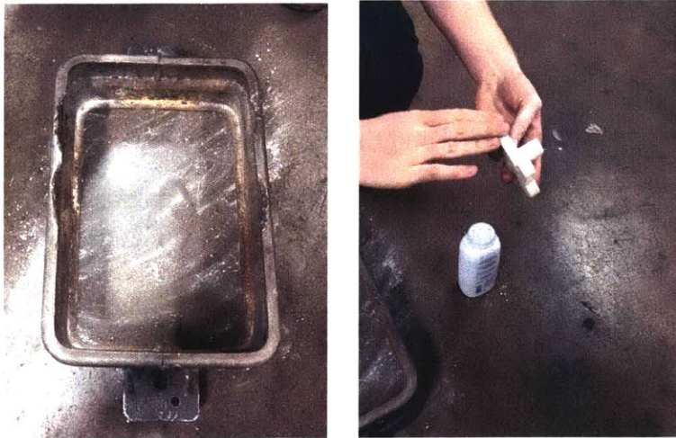
Figure 7: Cope is placed on the floor, top side down. The floor and pattern are powdered.
