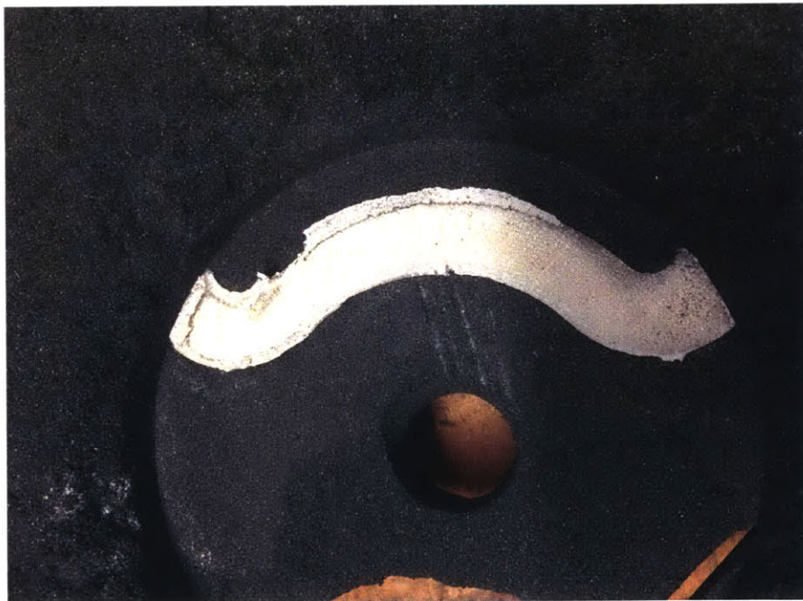
Figure 29: The moustache feature was stuck in the resin sand and broke off when the pattern was being removed from the shell.
