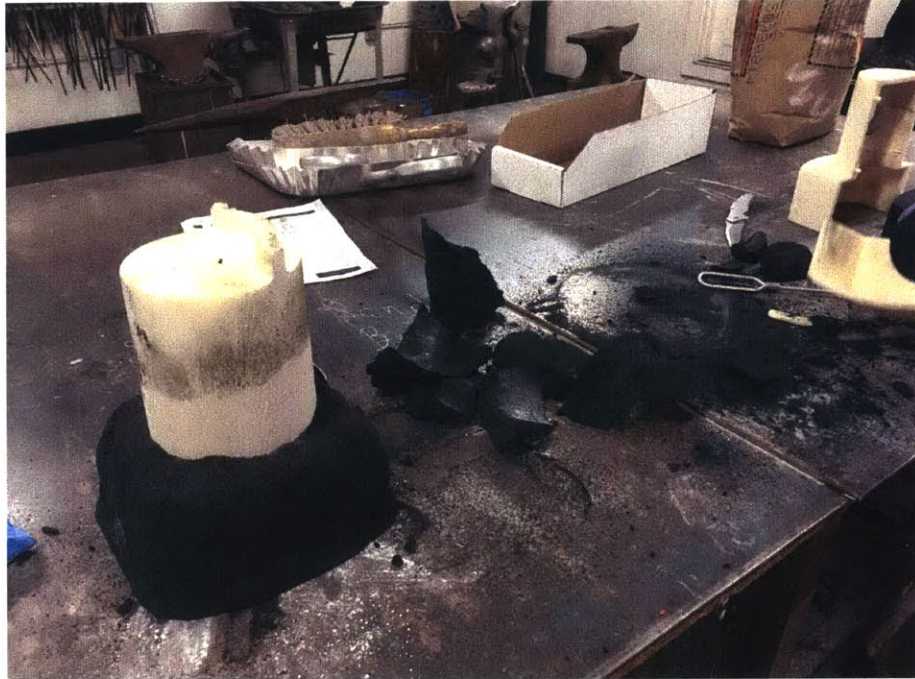
Figure 25: The shell broke apart only leaving the part surrounding the aligning feature intact.
