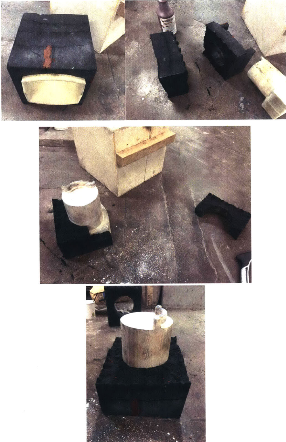
Figure 31: The shell casting of the piston fell apart at the boundary between resin sand layers. The first two layers were salvaged and only covered the alignment feature of the pattern.
