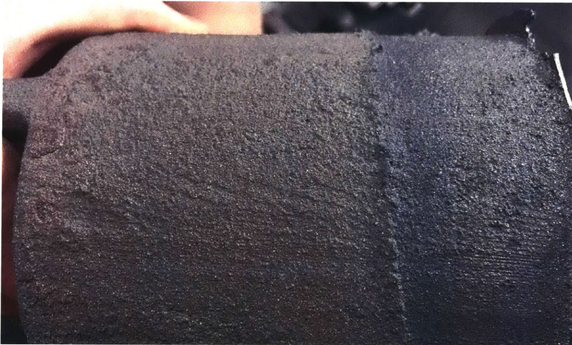
Figure 36: The difference in surface finish can be seen. The left side is where green sand met the pattern, the right side is where resin sand met the pattern.
