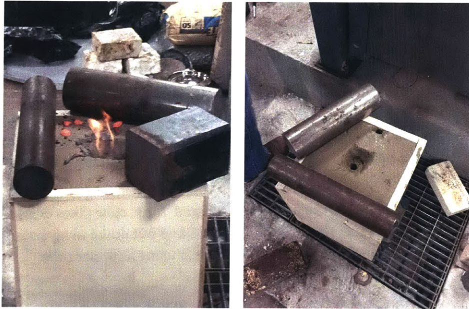
Figure 20: Molten iron is poured into the flask and flames appear from the top. The cast did not appear to fill fully.
