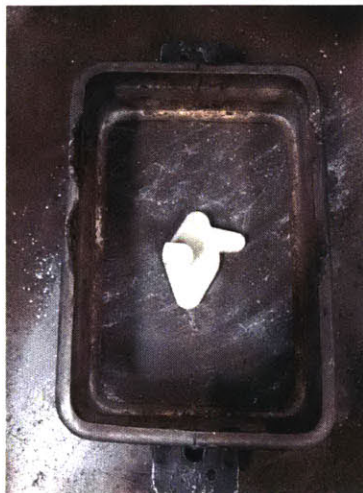
Figure 8: Top half of part is placed on the parting surface.
