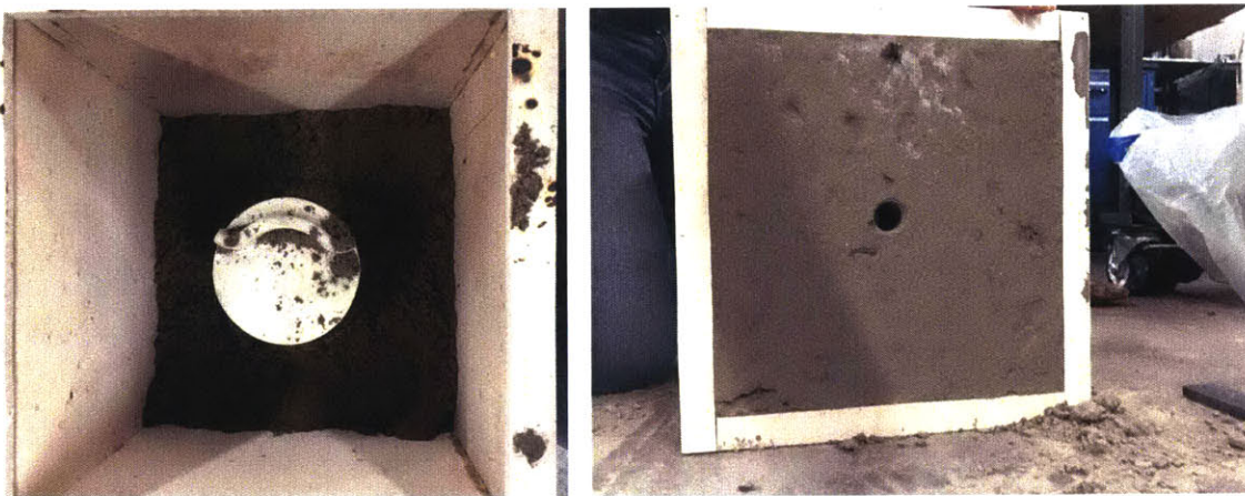
Figure 19: The piston pattern in placed in the flask and the flask is filled and rammed with sand.
