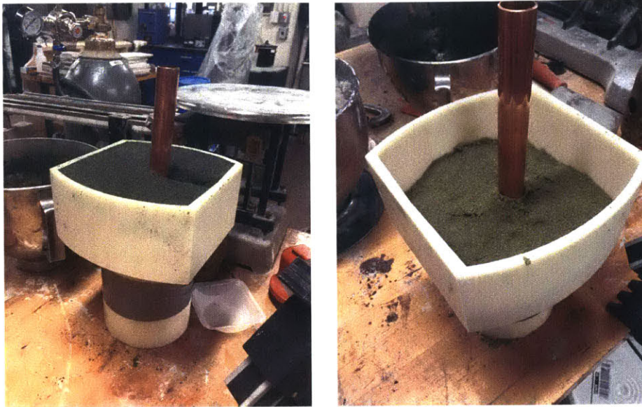
Figure 22: Second attempt at creating the core print. The mold is filled fully with sand using a copper tube to create a vent in the middle.
