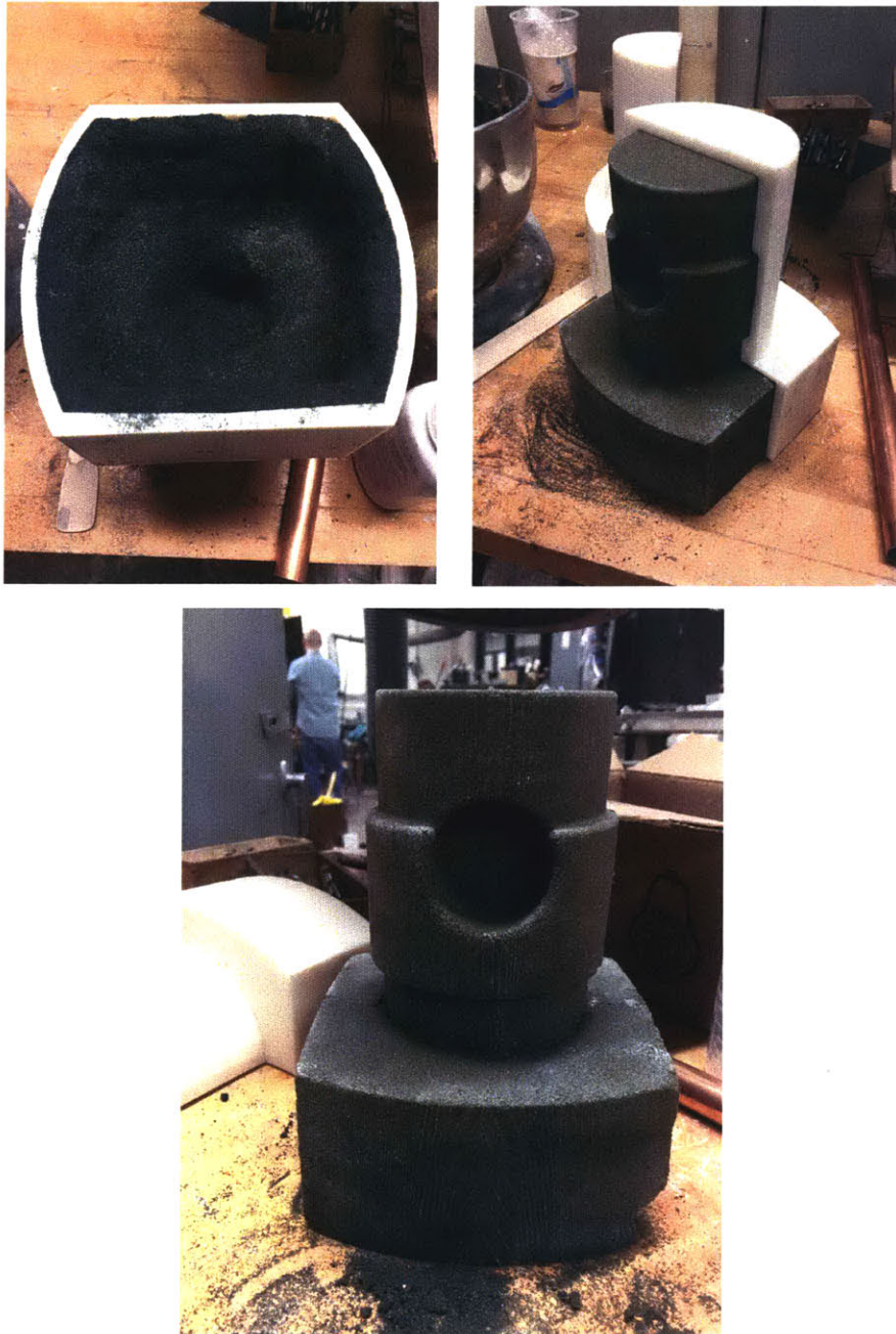
Figure 18: Core print made of resin sand, first attempt.
