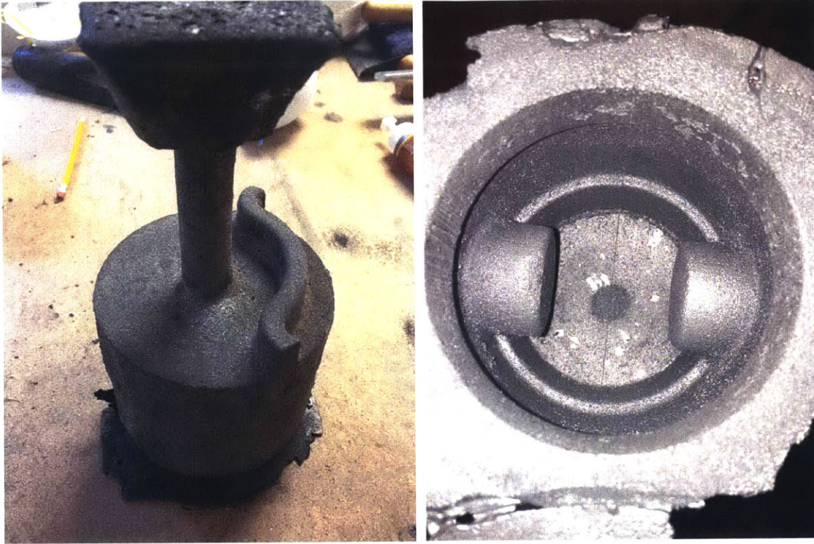
Figure 34: Full cast of the piston (left) and the cavity (right). The finish of the piston cavity is excellent.
