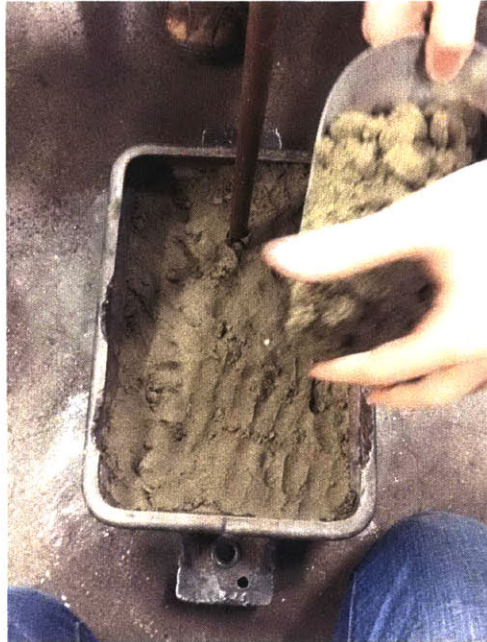
Figure 9: A dowel is placed to form the sprue and the cope is filled and rammed with sand in layers.
