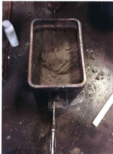
Figure 12: Drag is packed and rammed with sand.
