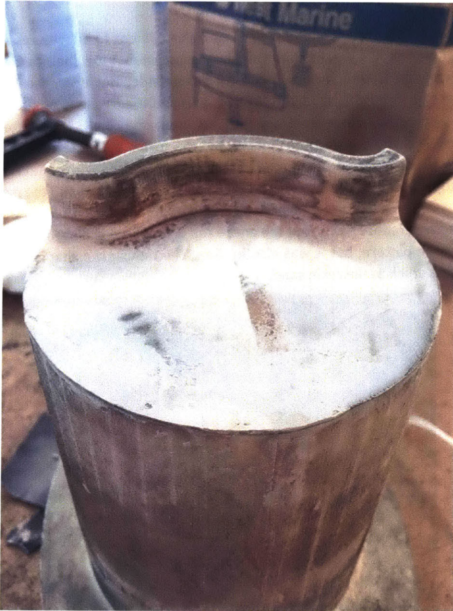
Figure 30: The moustache feature of the piston was epoxied to the pattern. The top was then plastered to fill in any holes and sanded to smooth out the surface.
