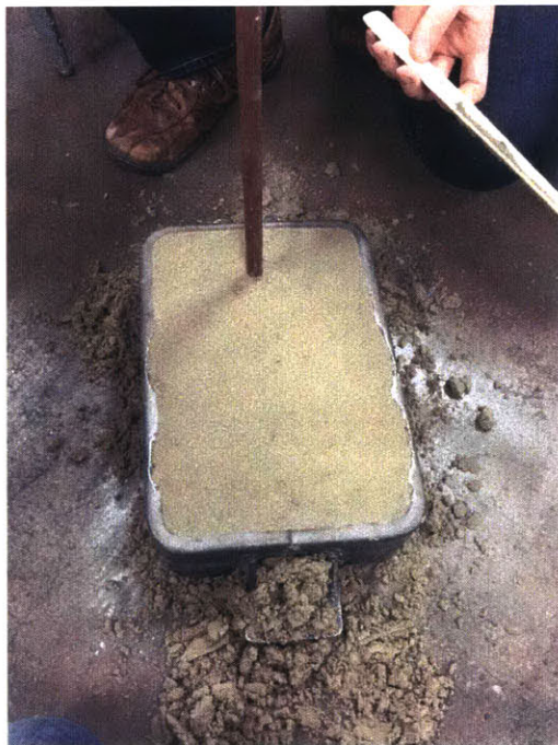
Figure 10: Once the cope is fully filled and rammed, a straight edge is used to scrape off excess sand.
