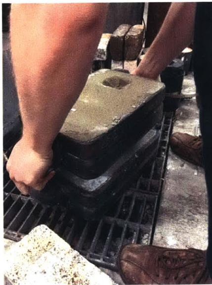
Figure 14: Cope is placed on top of drag and clamped prior to pouring.
