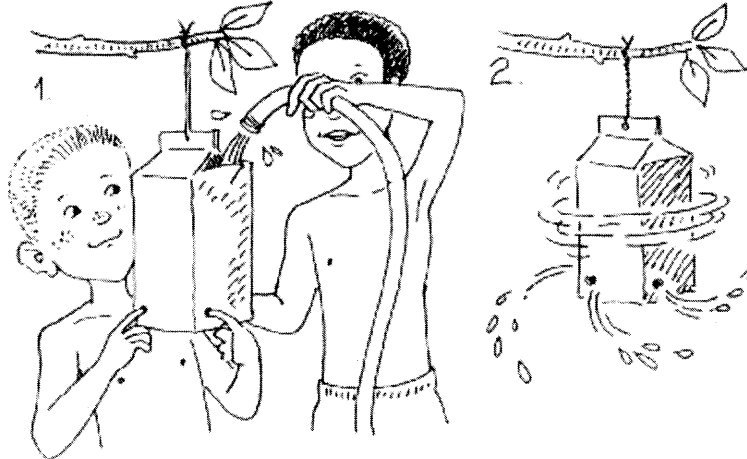
Figure 5-8 – Drawing of completed milk carton turbine hanging from tree Photo credit: Publications International, Ltd. (2007)
