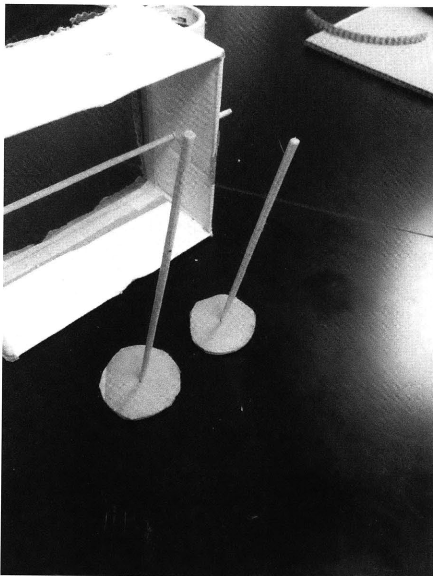
Figure 5-15 – Automata cardboard box assembly with cam shaft made of wooden skewer. Pushrod assembly consisting of two cardboard circles attached to two wooden skewers
