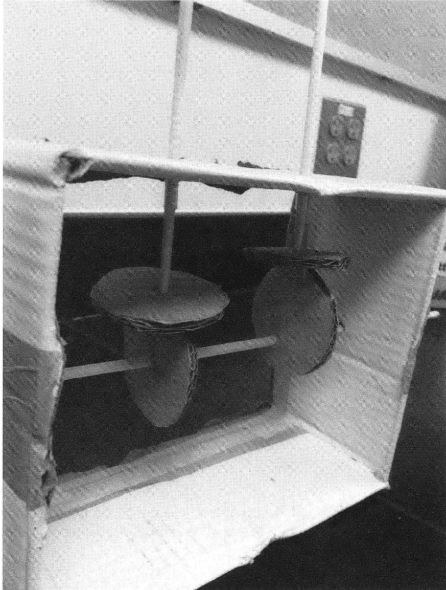
Figure 5-17 – Automata assembly consisting of push-rods and cam shaft made of wooden skewers, and circular cams made of cardboard
