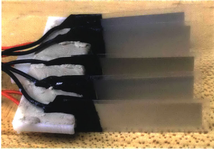
Figure 2-3: Clay used as an adhesive and for further support.
