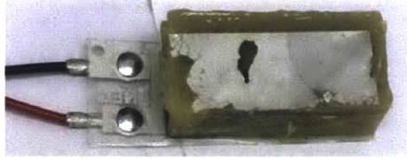
Figure 2-7: The residue of PVDF material after an attempt to detach the sensor from the spacer.
