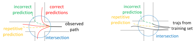
Fig. 7. Metric for evaluating prediction quality. Left: as a pedestrian enters an intersection, an algorithm makes predictions about the set of possible future paths the pedestrian may take. The predictions are evaluated by a hand-labeled set as ground truth. Right: poor predictions due to trajectory segments. Due to sensor occlusion, real datasets often contain fragmented trajectories, as shown in black. Predictions based on motion patterns (clusters) formed by fragmented trajectories can be repetitive (orange) or incorrect (green).
