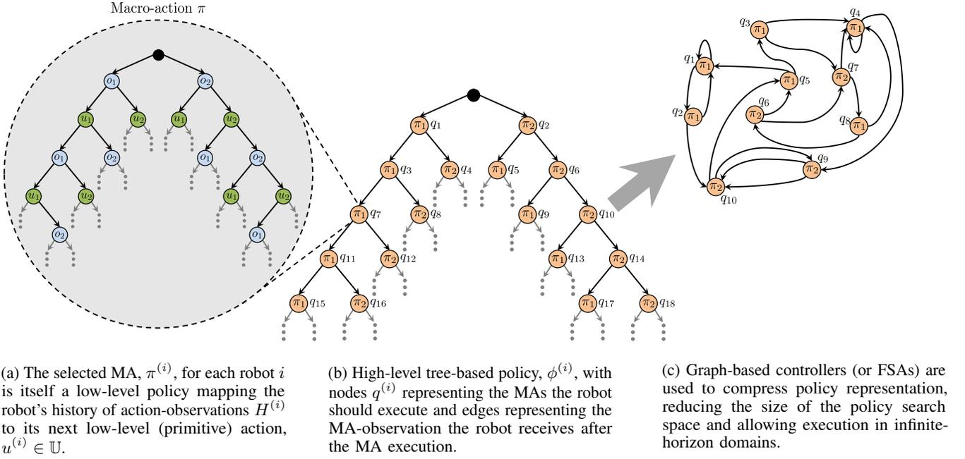
Fig. 1: Overview of hierarchical decision-making using the Dec-POSMDP. The above illustrates policy,  $\phi^{(i)}$ , for the  $i$ -th robot. Each robot's policy is represented as a high-level graph-based controller (right), which can be considered a compression of a tree-based policy over MAs (middle). Each MA is, in turn, a low-level policy (left).
