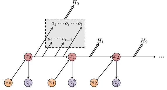
Fig. 2: Overview of the Dec-POSMDP sequential decision-making process. The  $i$ -th robot moves from state  $x_0$  through a sequence of MAs,  $\pi_0, \pi_1, \dots, \pi_k$ . Under each MA, it executes primitive actions  $u_1, \dots, u_{t-1}$  and perceives primitive observations  $o_1, \dots, o_t$ . At the end of each MA, it also obtains environmental observations  $o_0^e, \dots, o_k^e$ .
