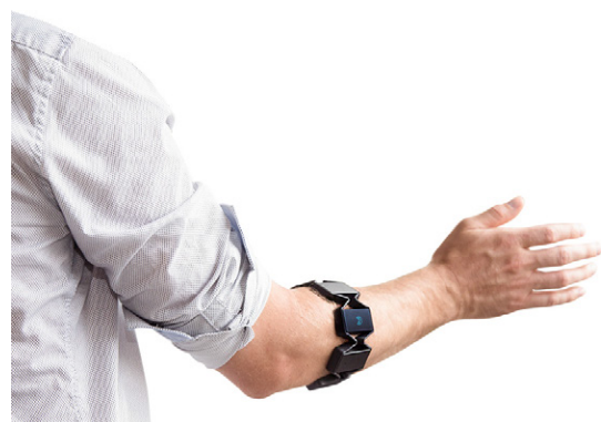
Fig. 34 MYO armband placed on forearm
