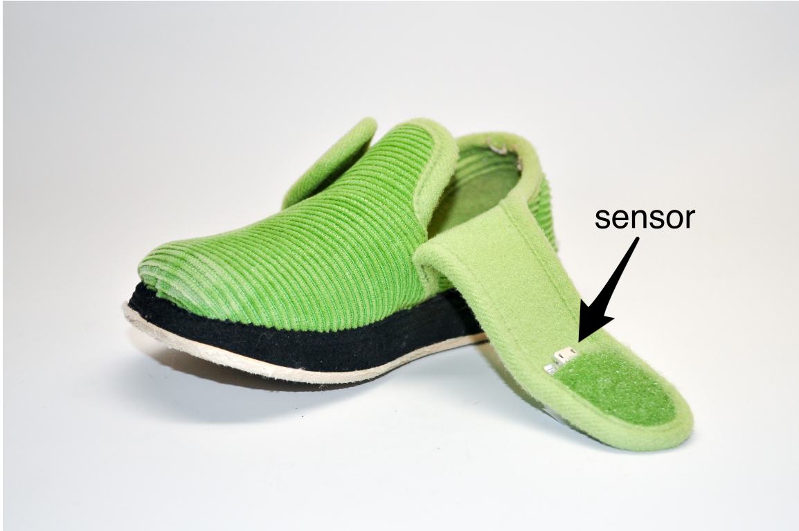
Figure 2-2: Sensors are placed in a minimally invasive way in the strap of the shoe.
