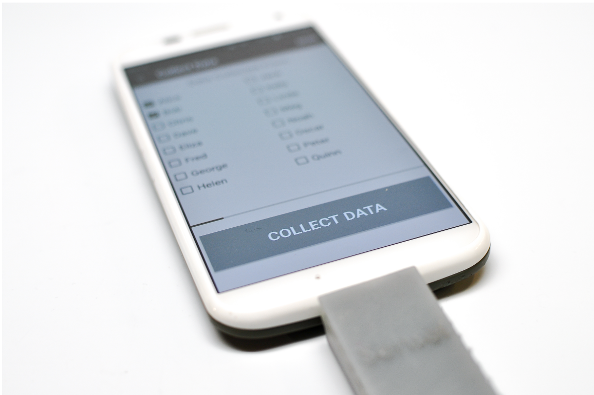
Figure B-5: The mother node sensor can be connected to the cellphone to start the sensors and collect data from the sensors.
