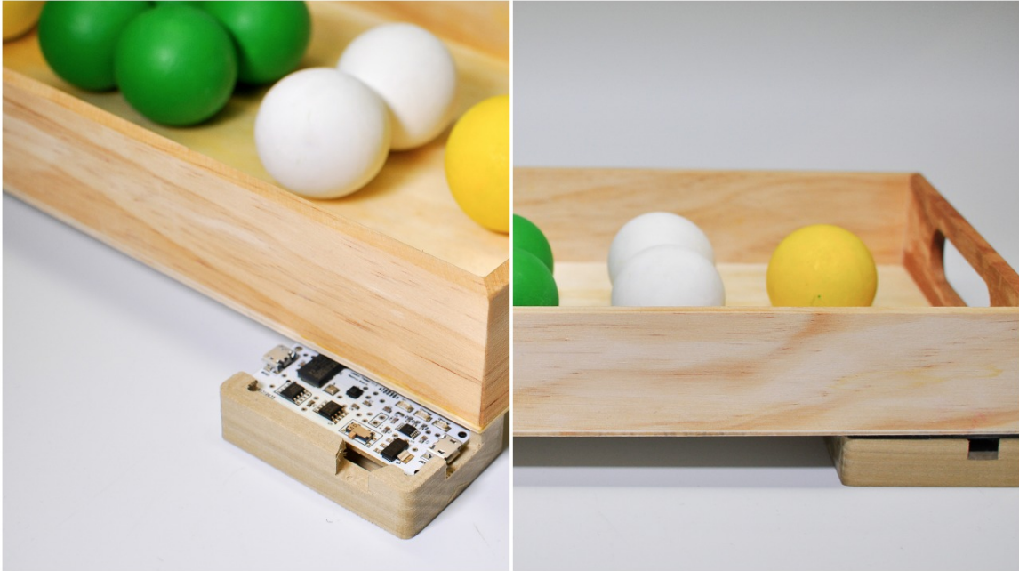
Figure B-4: Sensors can be placed in the feet of a lesson tray. These feet can be attached to any pre-existing lesson in the classroom.
