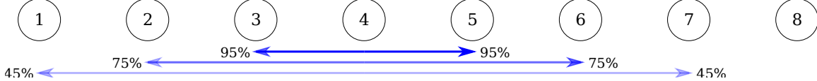
Figure 1-1: Linear mesh network with N = 8 nodes. The blue arrows represent a transmission from node 4. The transmission reaches nodes 3 and 5 with a probability of 95%, nodes 2 and 6 with a probability of 75%, nodes 1 and 7 with a probability of 45%, and node 8 with a probability of 0.
