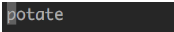
Figure 4-17: A screenshot of “potato.txt” with the file’s intended contents, “potate”. Since the array is allocated to the proper size before writing, the server does not write any nonsense.
