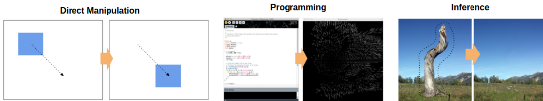
Figure 2-1: Examples of different types of tools for editing graphics, with mouse motion indicated by a dashed line. On the left is direct manipulation, in the middle is programming, and on the right is inference. Both programming and inference notably let users edit complex relationships, but it is often unclear to artists how actions will be realized on the graphic.
