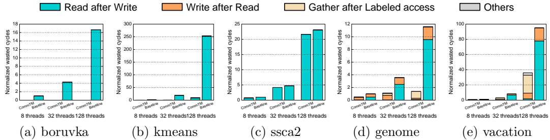
Figure 5-11: Breakdown of wasted cycles for COMMTM and baseline HTM for 8, 32, and 128 threads (lower is better).
