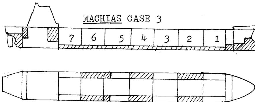
MACHIAS CASE 3: Double Bottom of depth 5.78 ft added to case 2 and the slop tank size is decreased.
