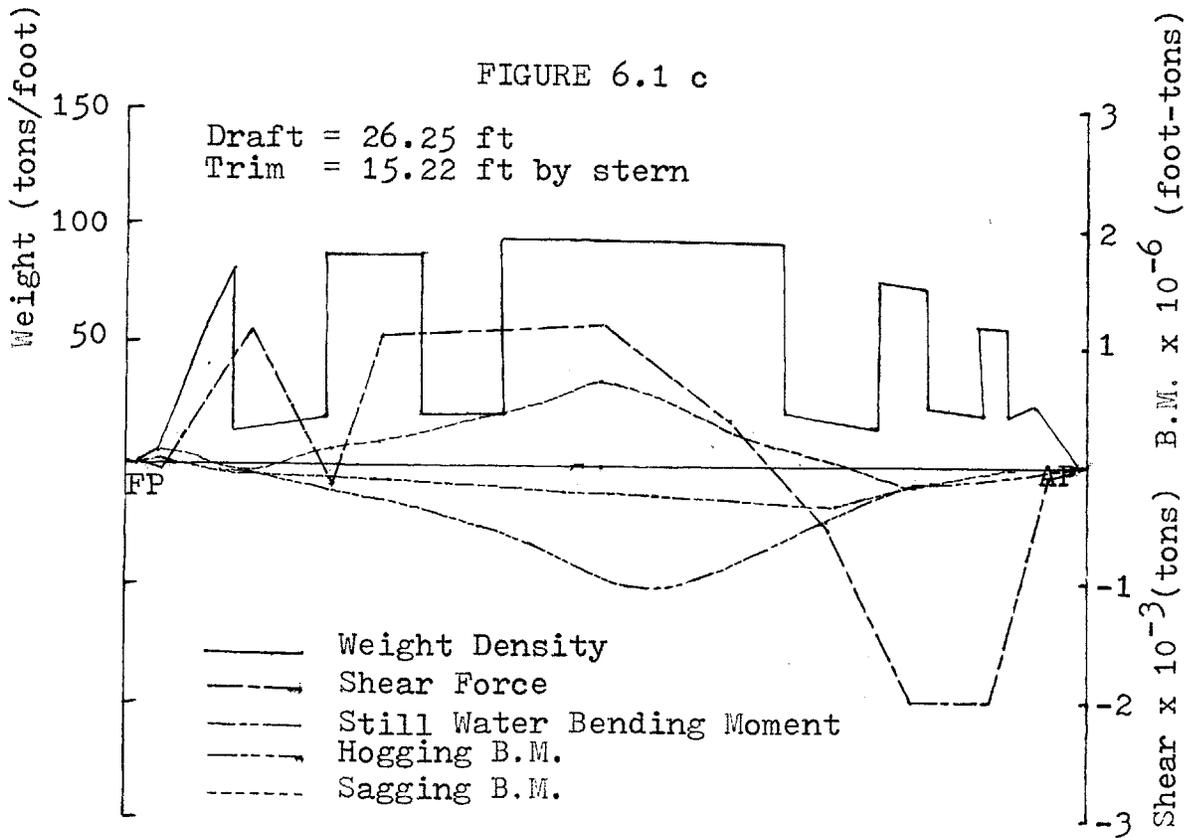
MACHIAS CASE 2: Longitudinal Bulkheads moved out 4.74 ft and slop tanks placed in Wkngs # 5.
