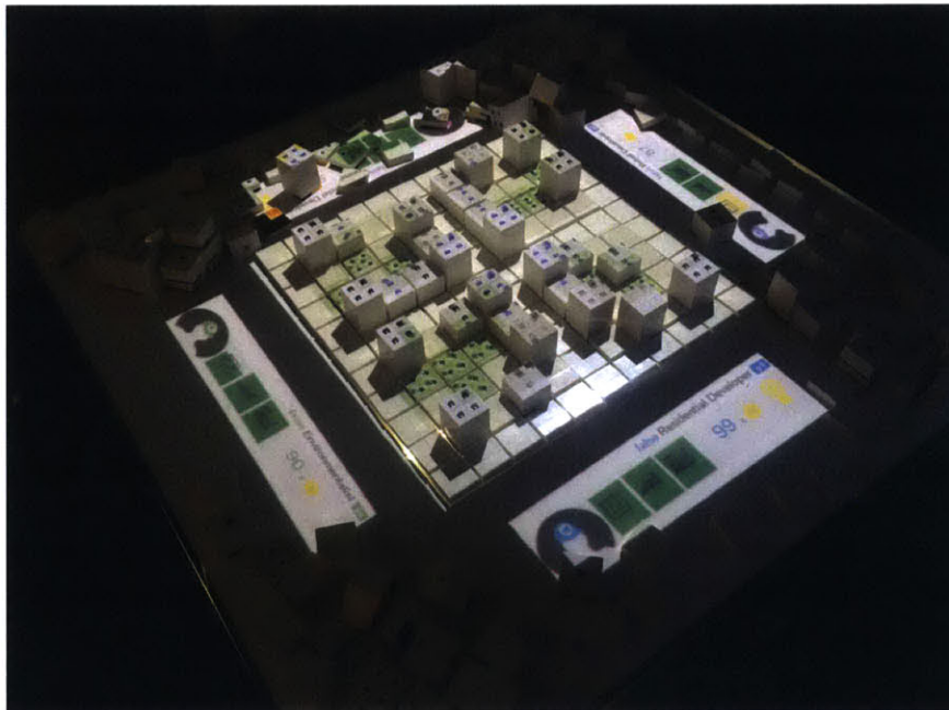
Figure 3-35: CityGame Tangible User Interface with boardgame, amenities and individual objectives visualized on the same game surface.
