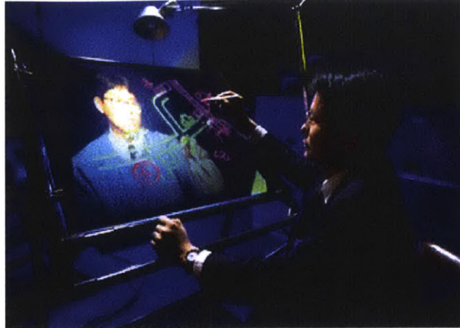
Figure 2-2: ClearBoard is a pioneering system supporting collaborative drawing in a shared space while seeing each other.
