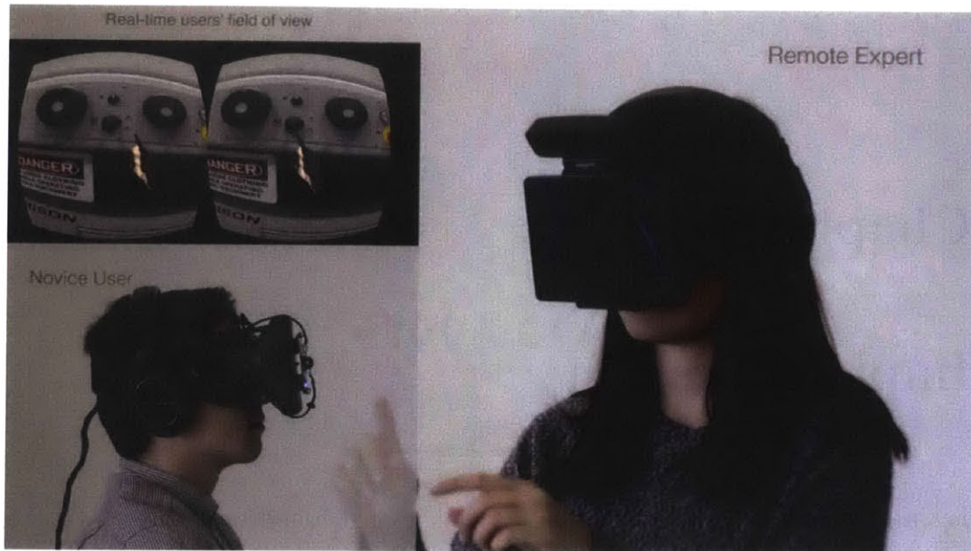
Figure 4-1: This figure shows users wearing the ShowMe++ system. Both the novice's field of view and the virtual hands are displayed in the figure.
