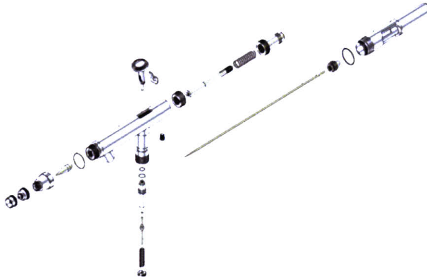
Figure 26 - Exploded view of the airbrush (image courtesy of Max Lieber)
