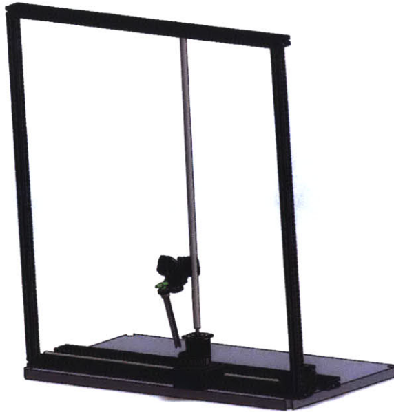
Figure 23 - The 8020 frame with X and Y stages in an inverted T setting
