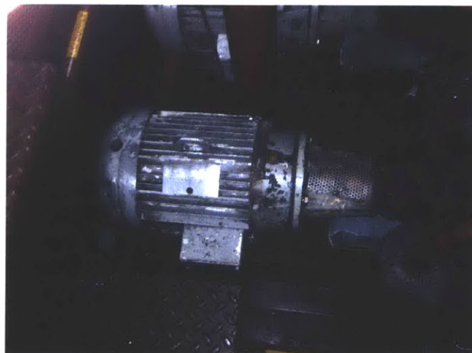
Figure 5-19: CPP "C" pump motor that supplies pressure to vary the pitch on the blades of the propeller. These pumps are energized when RMD is set and the vessel enters a time of increased risk and fatigue for the crew.
