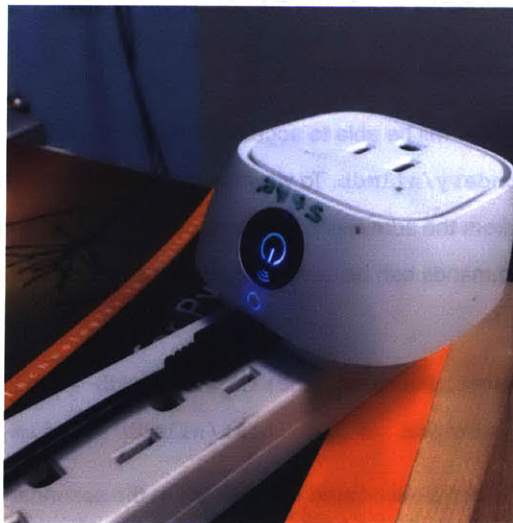
Smart Plug connected to a NILM by USB. Blue LED indicates an active USB communication between the NILM plug.
