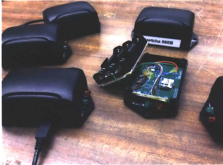
Figure 2-25: “Captcha” vibration diagnostic platform
