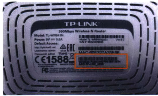
The default SSID and password are on the back of the router
