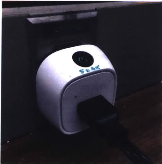
Smart Plug connected to a NILM over a wireless network. The green LED indicates the plug has authenticated to the network.
