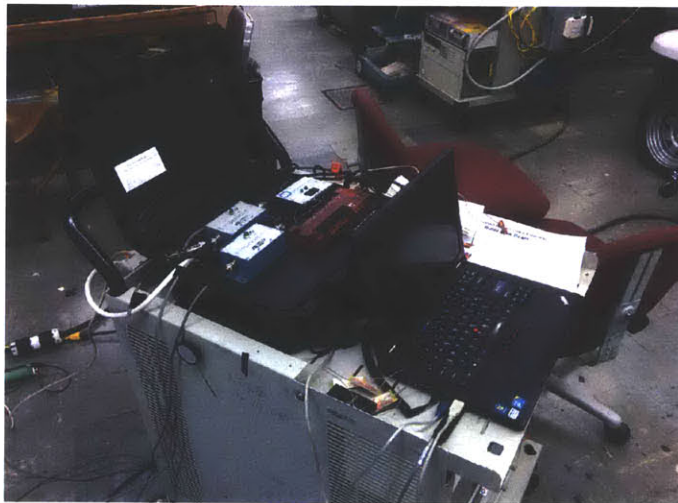
(b) Data Acquisition Blocks, Data Storage, and Power Supply and Wiring
