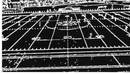
(a) Edges (shown as white) are extracted from the frame and dilated in width by factor of 2.
