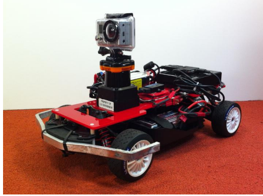
Figure 2: 1:8 scale RC car used in experiments, with Hokuyo laser range-finder, Microstrain IMU and computer.
