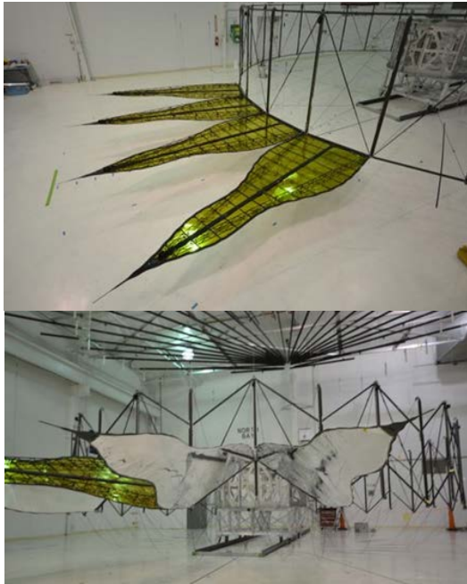
Figure 12. Deployed position tolerance demonstration. Petal root positions are measured after each of 20
