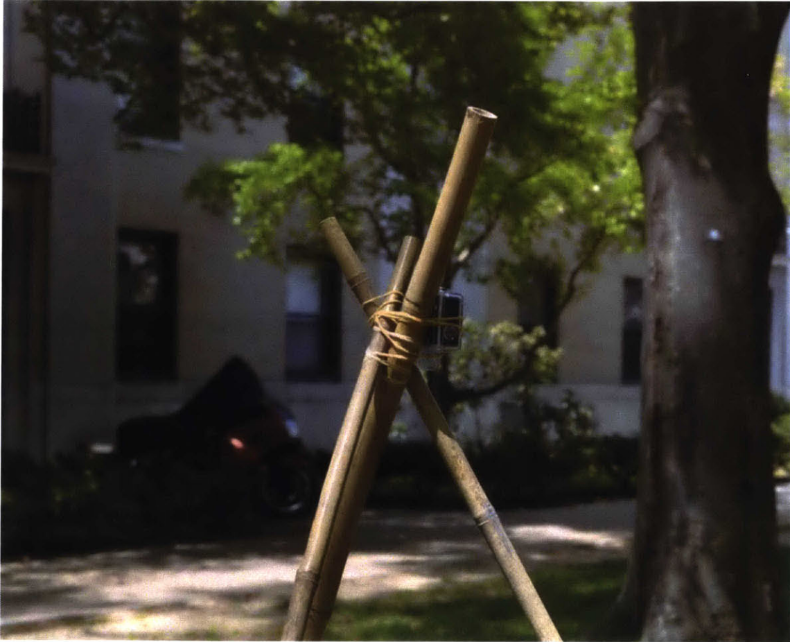
Figure A-1: The makeshift ‘tripod’ made of bamboo and rubber bands that was used to capture a time lapse of the building sequence.
