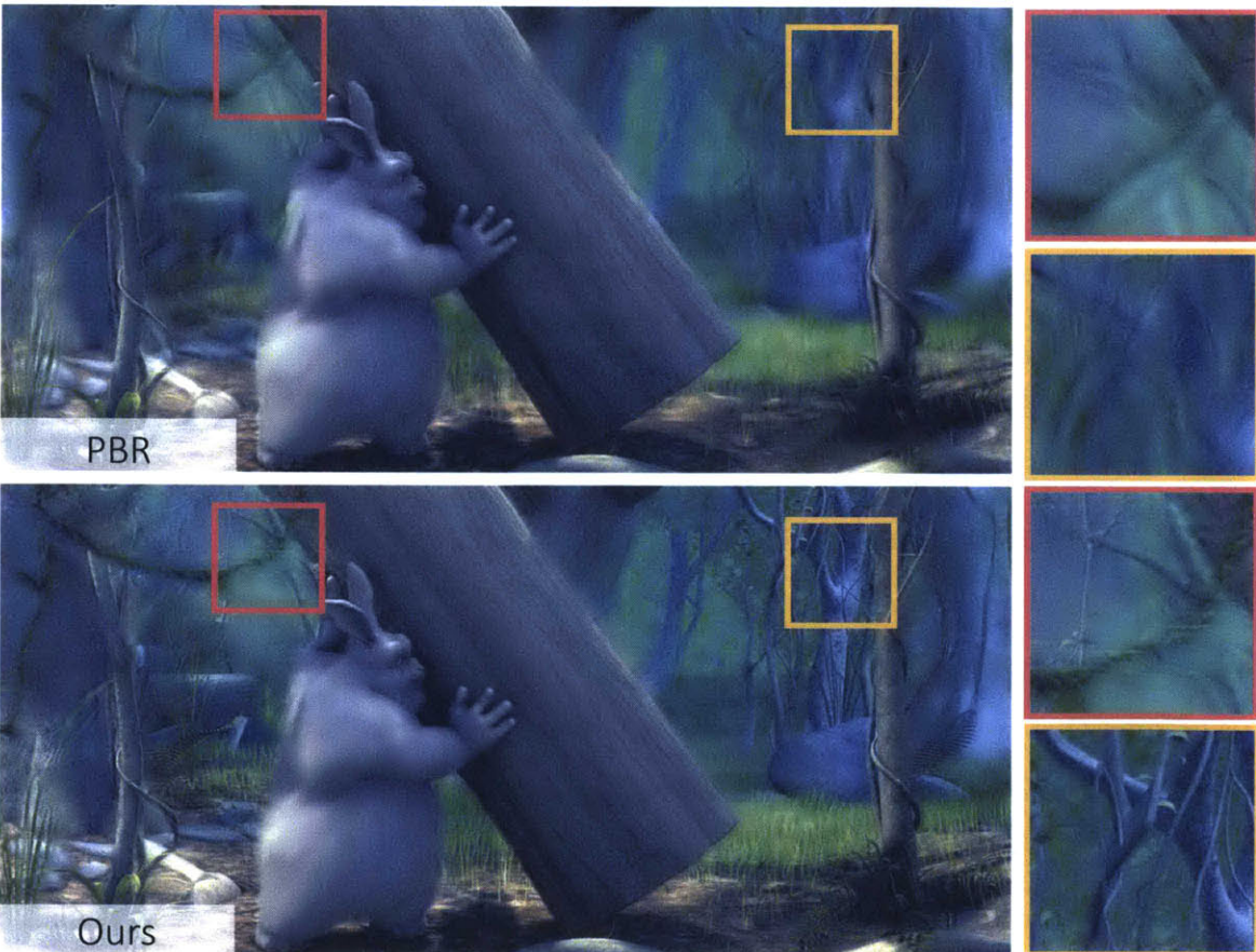
Figure 5-4: PBR approach cannot handle large disparities. As a result the higher frequencies are wrongly synthesized which leads to significant ringing and blurring. On the other hand, our method is able to correctly reproduce high frequency content and the synthesized image is much clearer.
