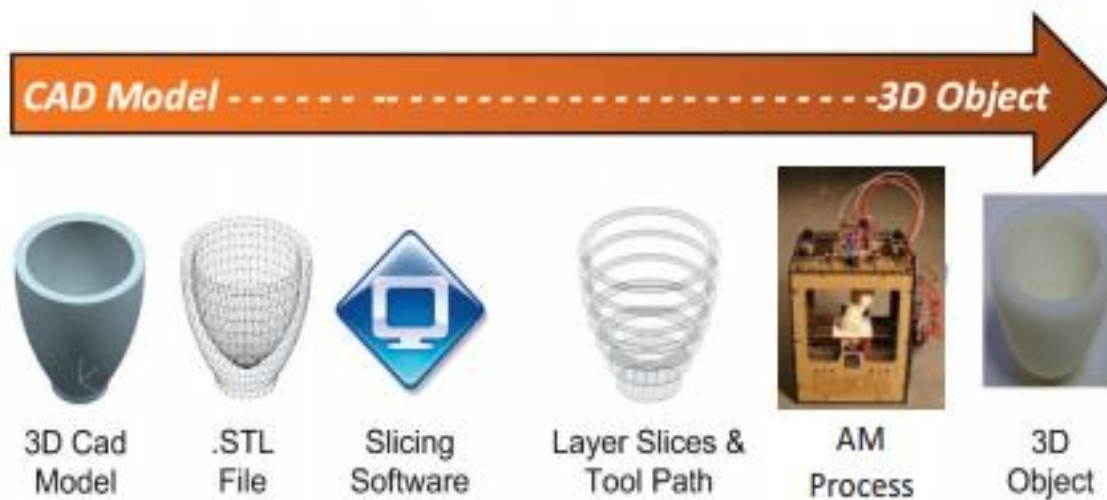
Figure 2-2: Generalized Additive Manufacturing Process [21]
