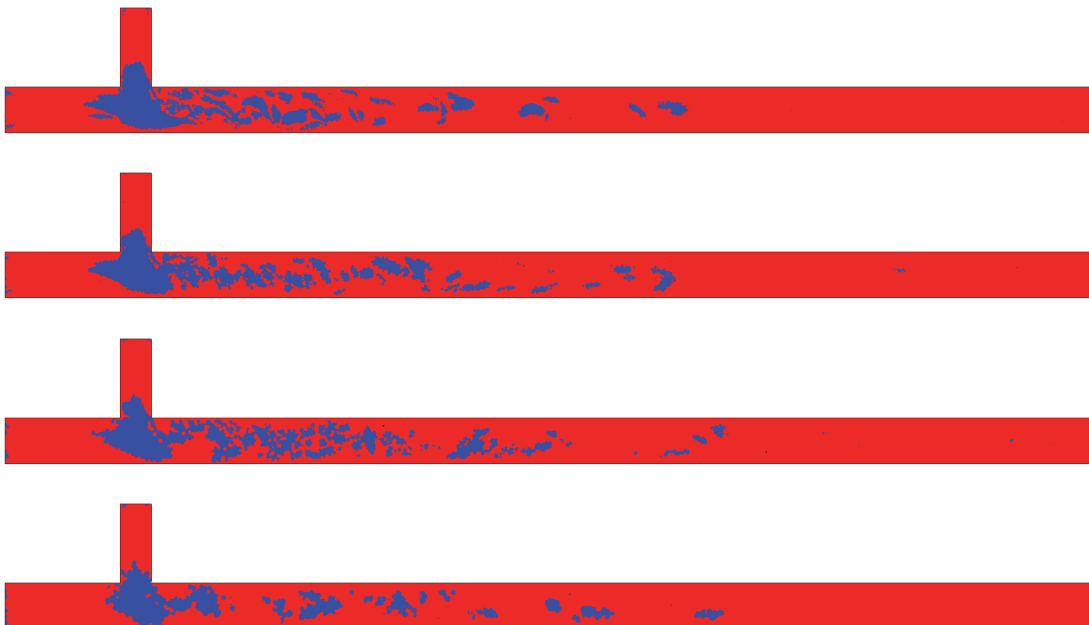
Figure 6.37 STRUCT activation regions for the four polyhedral grids of Table IX, ordered from the finest to the coarsest
