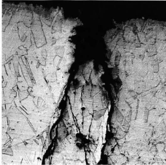
Figure 33: This image shows a crack that has initiated from a corrosion pit in stainless steel condenser tubes. The component was exposed to chloride-containing water, which induced pitting and chloride-assisted stress corrosion cracking. [43]
