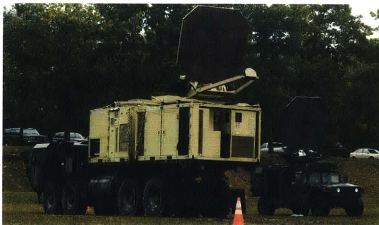
Figure 1-3: Photographs of current active denial systems mounted on vehicles for remote deployment that are in development by the US military [4].
