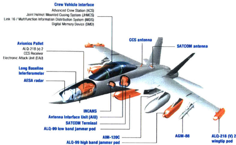
Figure 1-2: Schematic of the U.S. E-18G Growler jet, showing its armaments; a modified F/A-18, the Growler uses electronic warfare in place of bombs and missiles [3].
