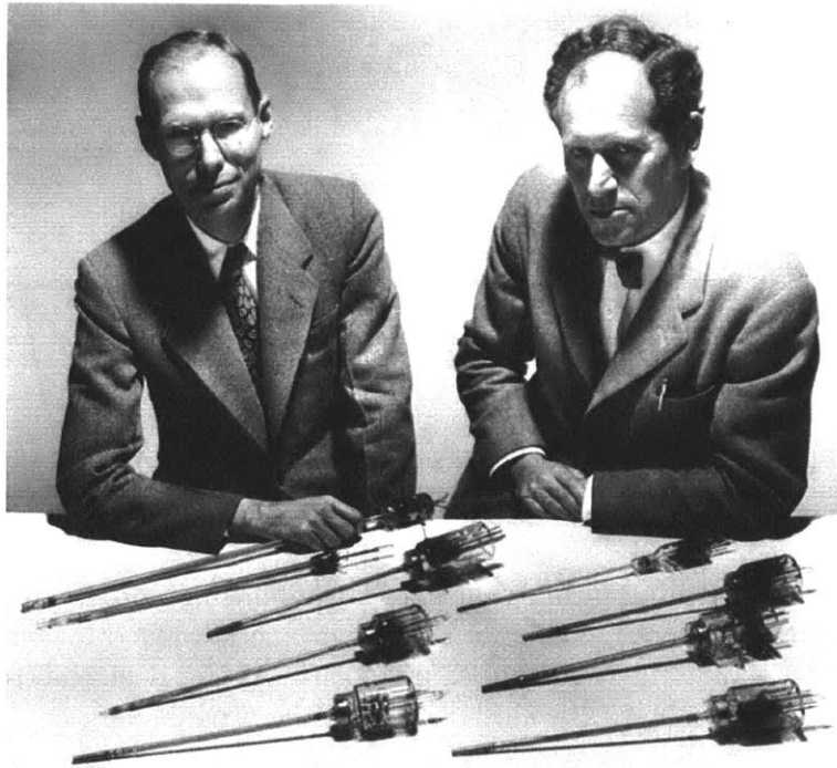
Figure 1-9: John R. Pierce (left) and Rudolph Kompfner (right) shown with some of their earliest TWT tubes. These tubes utilized a metal helix structure to slow down the electromagnetic wave in order to interact with the electron beam. These early tubes were enclosed in glass tubes in order to provide the vacuum necessary for the emitter of the electron gun to work. This photo was taken at Bell labs in the 1950's [25].
