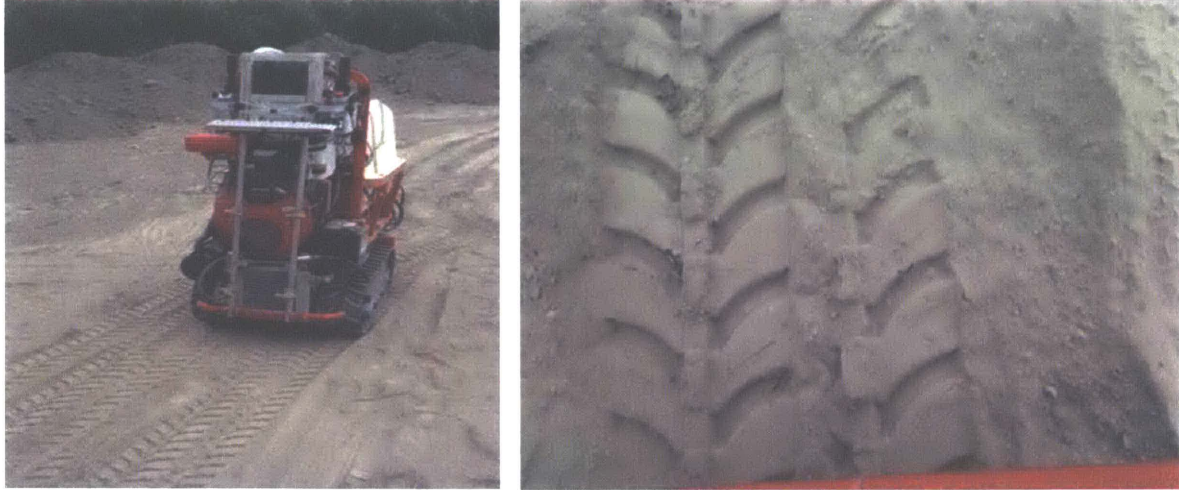
Figure 1.7. Figure of a tracked vehicle (left) and its track mark (right) [11]
