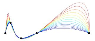
Fig. 2: Illustration of the iterative refinement of segment times, color-coded by total traversal time. The initial guess of total time is 10.5s (red) and the final optimized total time is 7s (blue).
