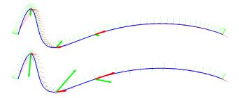
Fig. 3: Segment time optimization with the penalty on time  $k_T$  set at 500 (top) and 50000 (bottom). The optimal total trajectory times are 9.1s and 5.1s respectively. Vectors for waypoint velocity (red) and acceleration (green) are shown.
