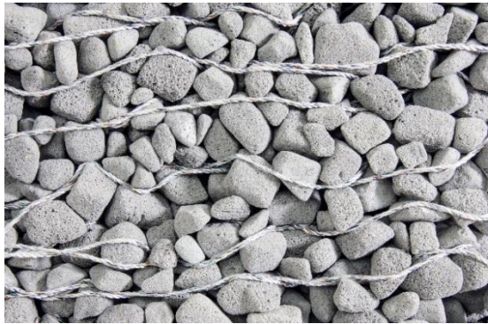
Fig. 14 Close up of a jammed structure, showing the string preventing the buckling of the force chains at the edge condition. Gramazio Kohler Research, ETH Zürich, 2014
