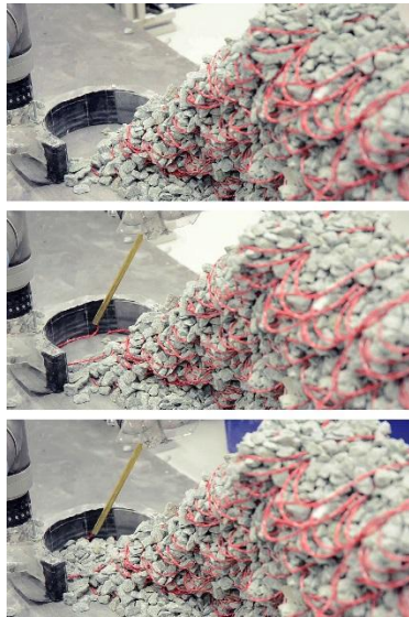
Fig. 12 Sequence of the fabrication process showing two six-axis industrial robotic arms equipped with customized end-effectors that cooperatively manipulate crushed gneiss and position textile strings according to a digitally generated weaving pattern. This is used for the robotic extrusion of textile strings that provide the lateral tensile support needed for preventing the buckling of the force chains and to stabilise the boundary fragility of the jammed structure (picture interval approx. 30 s.). Gramazio Kohler Research, ETH Zürich, 2014.
