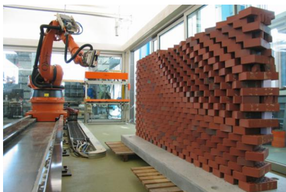
Fig. 4 Detail view of a dry-stacked automatically fabricated brick wall [19] together with a robotic setup equipped with a custom end-effector. Gramazio Kohler Research, ETH Zürich, 2006.
