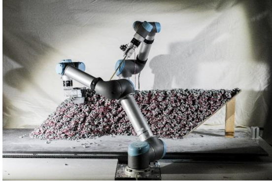
Fig. 13 The resulting robotic aggregation (1:5 scale) features considerable geometric capabilities – suitable to building construction purposes – and demonstrates that jammed architectural structures have the potential to be robust tectonic elements. Gramazio Kohler Research, ETH Zürich, 2014.
