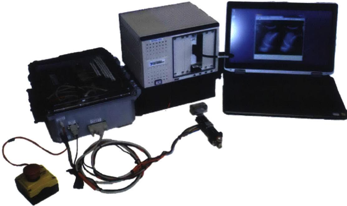
(a) The force controlled acquisition setup
