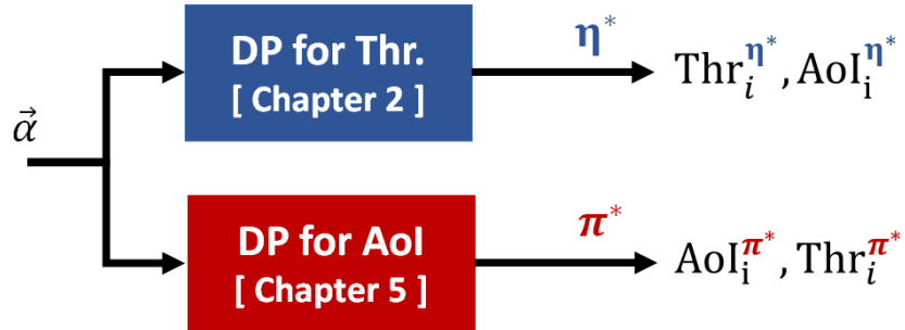
Figure 5-6: Diagram that represents the comparison between AoI-optimal policies and throughput-optimal policies. For each fixed \vec{\alpha} , four vectors are obtained, one for each combination of metric and policy. One example of such vector is (\text{AoI}_i^{\eta^*})_{i=1}^N .
