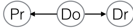
Figure 4-2: An illustration of relationship between the three entities in KDD cup 2014: Projects (Pr), Donations(Do) and Donors (Dr). Projects have a backward relationship with donations (since a project may have multiple donations), a donor has a backward relationship with donations (since a donor can be associated with with multiple donations).
