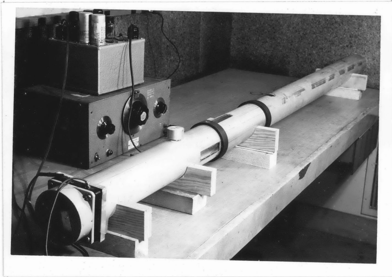
Figure 23 : Photograph showing the driver section, test section and termination section set up for making travelling wave observations.
