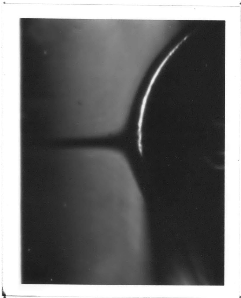
Figure 16 a,b : A photograph and schematic sketch of the streaming flow for R = 75 , s/a = .036 . The bright line indicates the edge of the cylinder. The double arrow in the schematic indicates the direction of oscillation. The exposure was 2 seconds on Kodak Super XX film.
