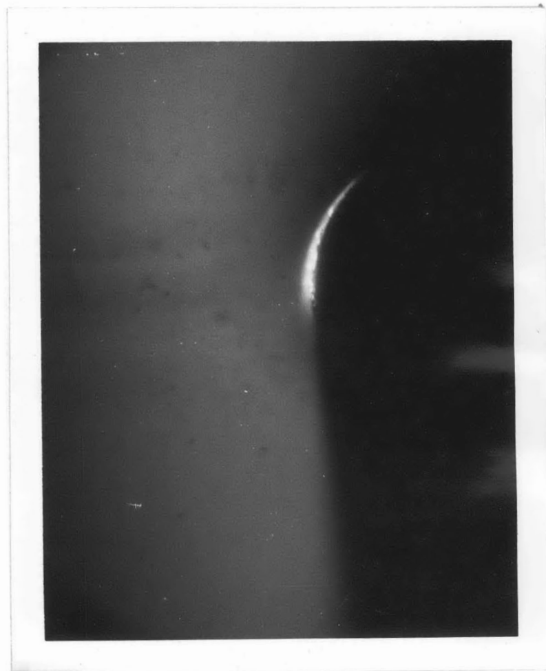
Figure 20 a,b : Photographs indicating the flow pattern before and after the inner boundary layer circulation is squeezed out and carried away. ( The flow is similar to that in figure 16 a,b in direction and nature.) The squeeze out occurs for R = 270 , s/a = .55 . The exposure was 2 seconds on Super XX film.
