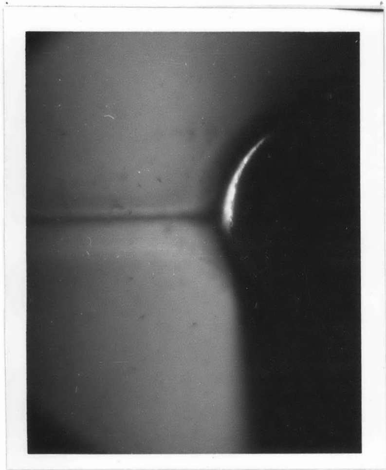
Figure 20 a,b : Photographs indicating the flow pattern before and after the inner boundary layer circulation is squeezed out and carried away. ( The flow is similar to that in figure 16 a,b in direction and nature.) The squeeze out occurs for R = 270 , s/a = .55 . The exposure was 2 seconds on Super XX film.
