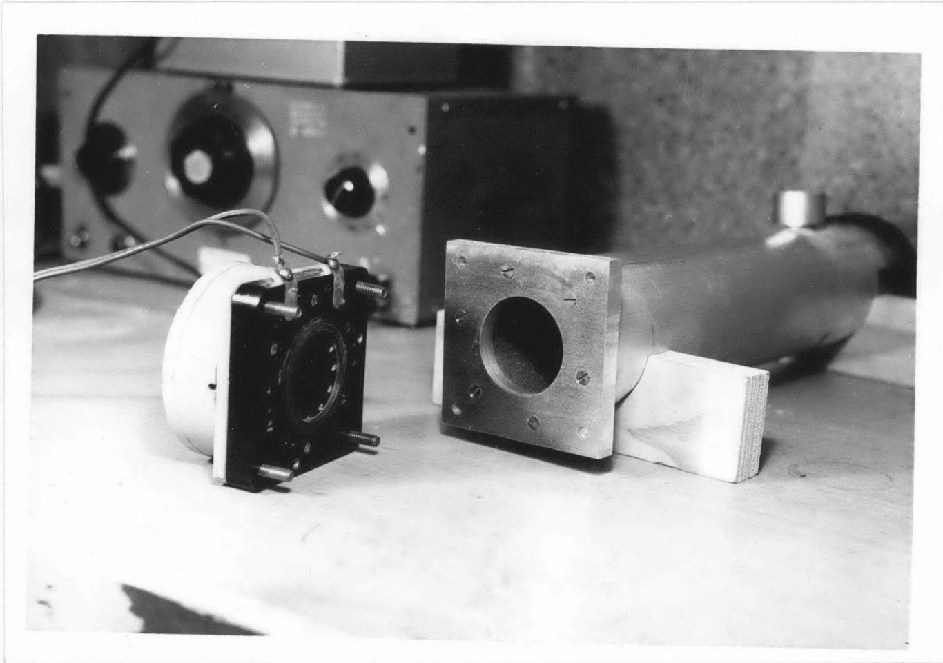
Figure 25 : Photograph showing the speaker unit and the fitting with which it is coupled to the driver section.
