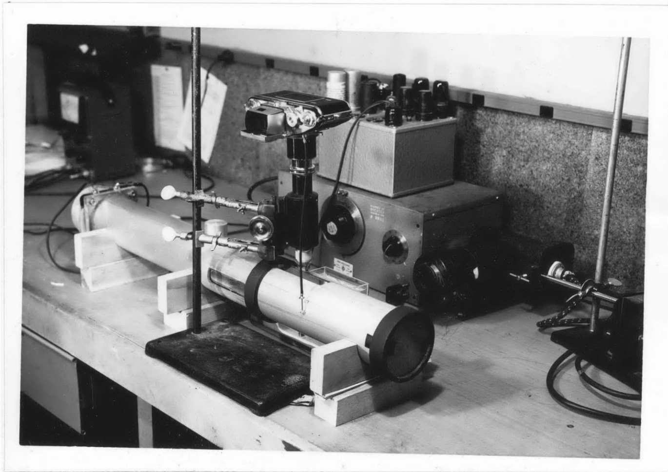
Figure 21: Photograph showing the standing wave tube in which the streaming motions were observed. The camera and microscope arrangement is set up ready for taking photographs of the flow. The light source, amplifier, and audio oscillator are also shown.
