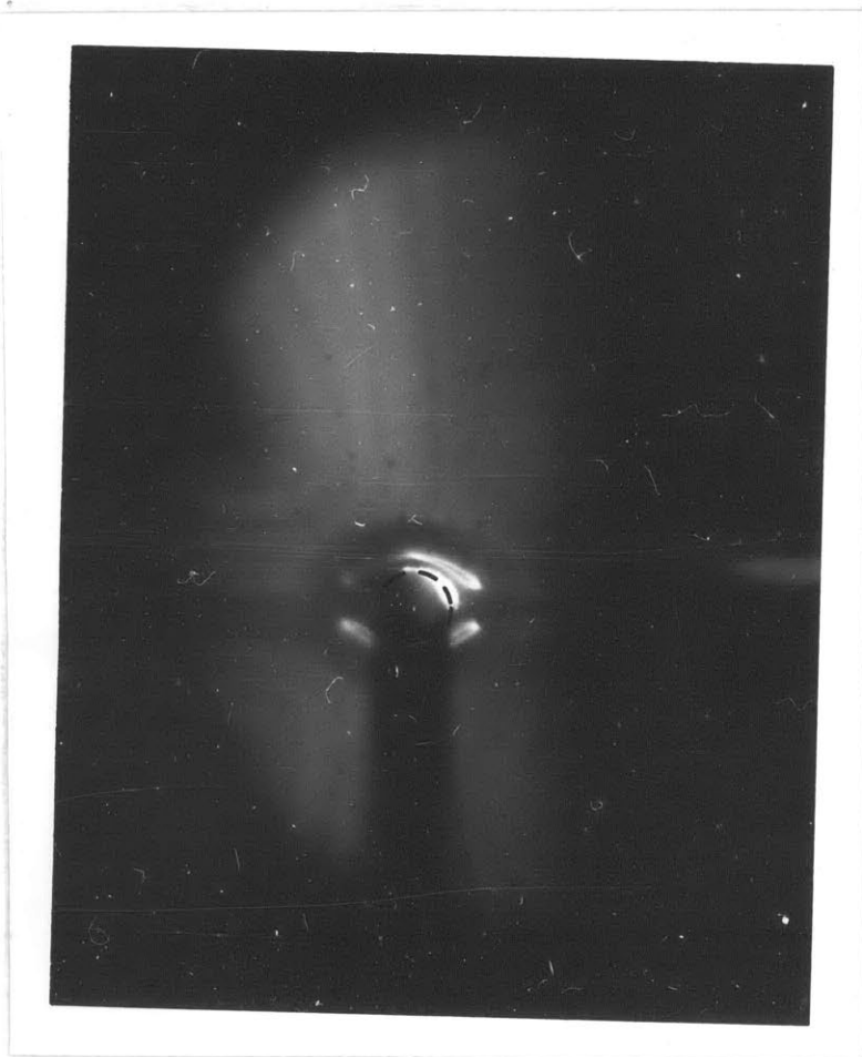
Figure 17 a,b : A photograph and schematic sketch of the flow for R = 20 , s/a = .65 . The edge of the cylinder is indicated by the dotted line on the photograph. The double arrow in the schematic indicates the direction of oscillation. The exposure was 2 seconds on Kodak Super XX film.
